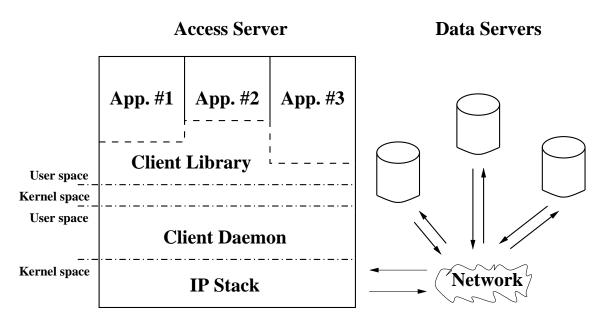
Figure 1: Process Architecture Sketch
